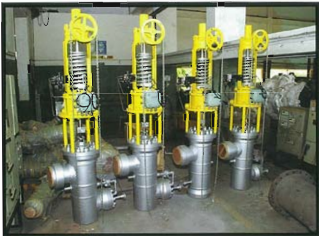
PRDS Systems for L&T - IOCL Panipat plant
