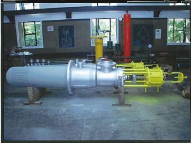
HP Bypass valve along with Dump Tube
