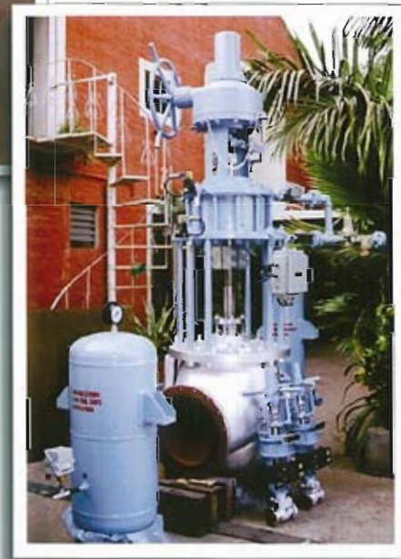
16" size On/Off Control valve supplied to Khanna Paper. Valve opened in 0.5 secs and was supplied with air receiver and other instruments as a complete package.
