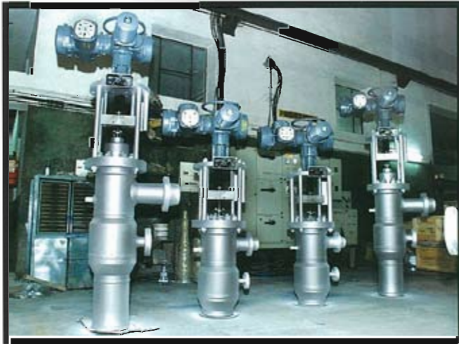
HP & LP Bypass valves for Atomic power plant
