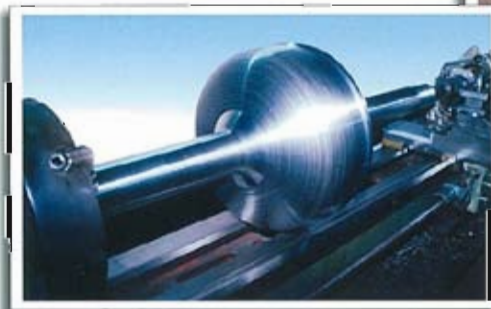
Machining of 20" size plug being carried out at in-house facility
