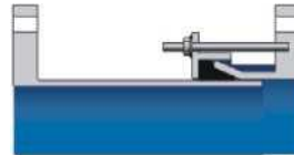
Unrestrained Dismantling Joint
