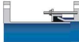
Unrestrained Dismantling Joint
