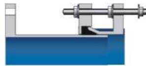
Unrestrained Dismantling Joint
